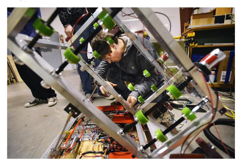
Staff photo by E.J. HarrisSophomore Landon Thornburg works on mounting a sprocket for a drive system on the robot
